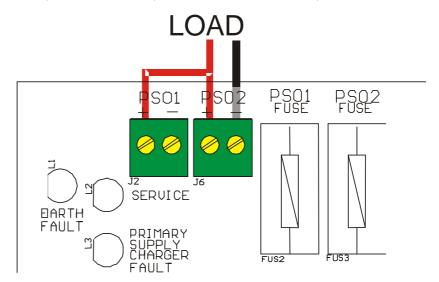
The negative is common in the control board and thus does not need to be bridged.
