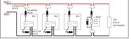
Note: If non-polarised alarm devices (eg some types of old mechanical bell, or a relay) are used, then a diode will have to be placed in line with the device to enable fault monitoring. They may also need a
