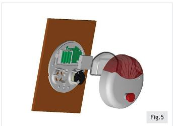
It can be installed on boards, walls or wherever it can be hung (these should be places where the unit is easily visible). Fix the screw according to figure 4 and complete the installation according to figure 5.
