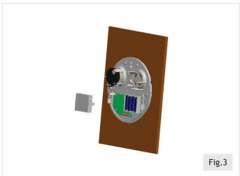
Install batteries as shown in figures 2 & 3 above (note that the battery sign is shown on battery box).
