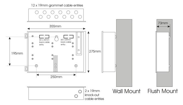
Fix the enclosure to the wall using the three mounting holes provided.
