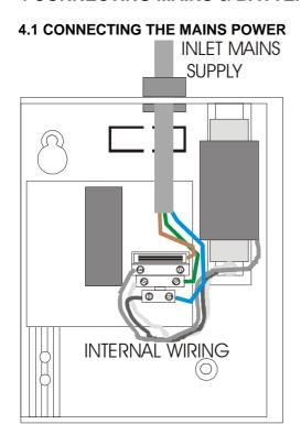
The panel should be connected to 220-240V AC by a 3A rated spur to the fuse box with 1mm<sup>2</sup> to 2.5mm<sup>2</sup> 3-core cable. Nothing else should be connected to this supply. This cable should be fire resistant.
