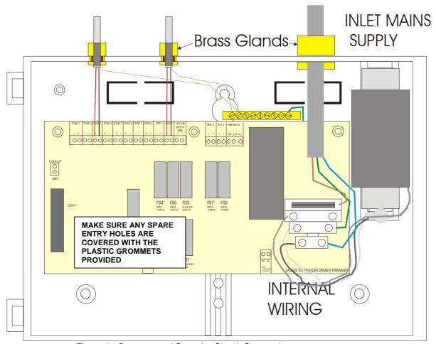
Figure 6: Detector and Sounder Circuit Connection
