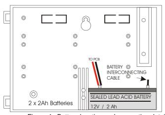
Figure 4: Battery location and connection details
