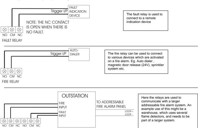
The termination for the above inputs must be as indicated on the main PCB (See page 15). The Earthing of the cable screens should be as shown on page 9.
