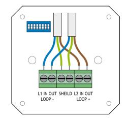
The loop +, loop -, and loop screen cables connect to terminals on the sounder PCB.
