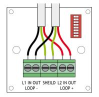
The loop +, loop -, and loop screen cables connect to terminals on the sounder PCB.
