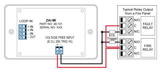
The end of line resistor value is  $20 \text{K} \Omega$  and the trigger resistor value i.
