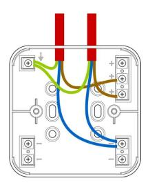
Connecting the sounder is done using the terminals in the back box of the device. Please refer to the above diagram.
