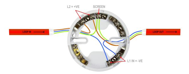
The connection for the detectors bases is made as follows:
