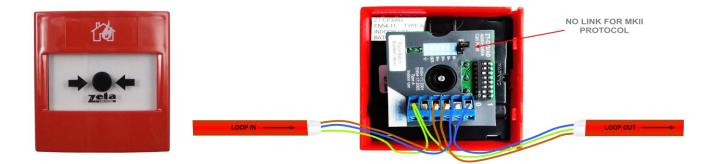
The CP3/AD call point has a built in isolator which can be wired in circuit or not used. This is done by means of not wiring to the negative out terminal on the call point. The following terminals are used for connecting the call point.
