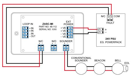
The ZASC requires a external 24vdc power supply (as shown in the above diagram). The EOL for the sounder circuit is  $10K\Omega$ . When using the ZASC make sure the PSU being used has a fault output relay, so that in the event of a power supply fault it is reported to the control panel.
