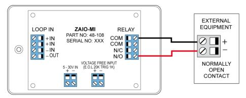
The end of line resistor value is  $20 \text{K} \Omega$  and the trigger resistor value is 1 K
