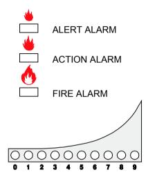
BARGRAPH of SMOKE LEVEL or AIRFLOW SPEED
