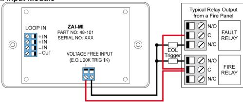
The end of line resistor value is  $20K\Omega$  and the trigger resistor value is  $1~K\Omega$ .
