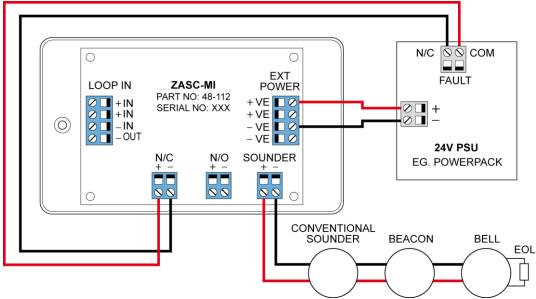
The ZASC requires an external 24vdc power supply (as shown in the above diagram). The EOL for the sounder circuit is  $10K\Omega$ . When using the ZASC make sure the PSU being used has a fault output relay, so that in the event of a power supply fault it is reported to the control panel.
