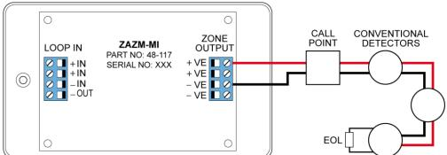
The ZAZM powers the conventional zone from the addressable systems loop, so no external power supply is required. The EOL for the zone is  $6.2K\Omega$ .
