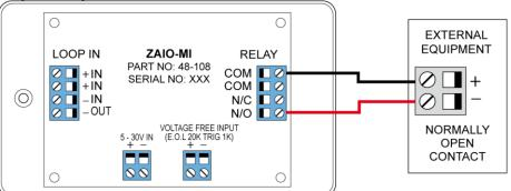
The end of line resistor value is  $20K\Omega$  and the trigger resistor value is 1K
