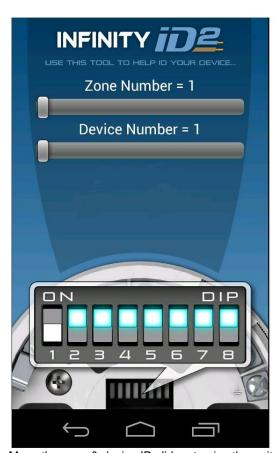
Move the zone & device ID sliders to give the switch settings for each device
