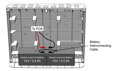
Figure 4: Battery location and connection details
