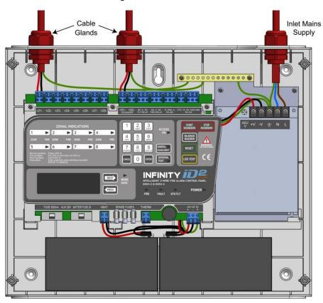
All cables entering the enclosure should have cable glands, which will prevent unwanted openings in the enclosure.
